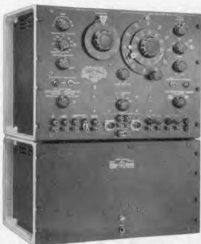
Figure 1B. View of the complete Pulse, Sweep, and Time-Delay Generator, with power supply.
